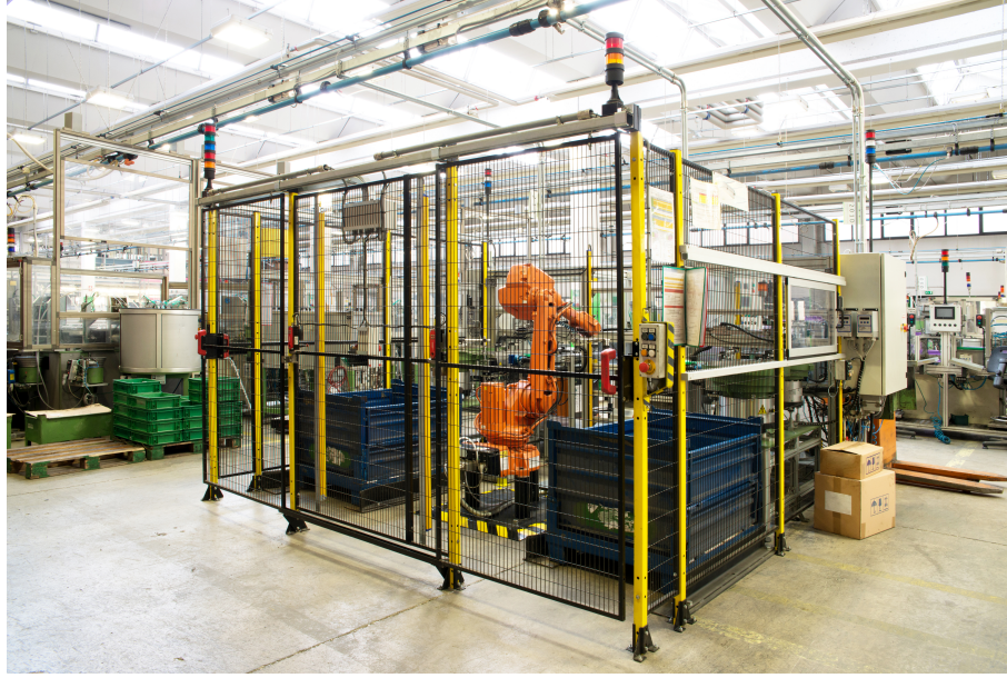
Figure 1.1: Industrial robot kept in a cage to prevent injuries from humans.
